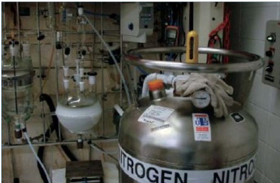
Albemarle uses liquid nitrogen cooling on this 10-litre, low temperature laboratory apparatus
